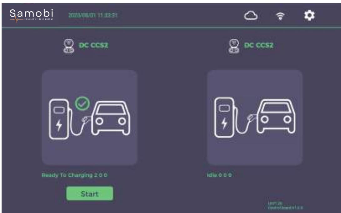
3. To change the charging mode, you need to access the settings interface. The user password for the settings interface is initially set to 'No Password'.
