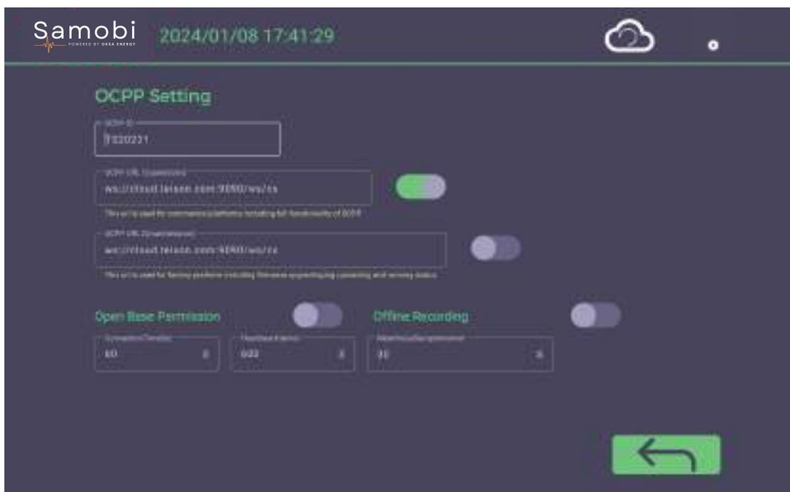
A. Cloud platform connection supports dual platform simultaneous connection. UL1 has functions such as remote control of charging stations, access to charging logs, charging data, charging status, and remote firmware upgrades; UL2 only supports remote firmware upgrade, access to charging logs, and access to charging status. (UL2 connection platform function, UL1 platform must be turned on to work)
