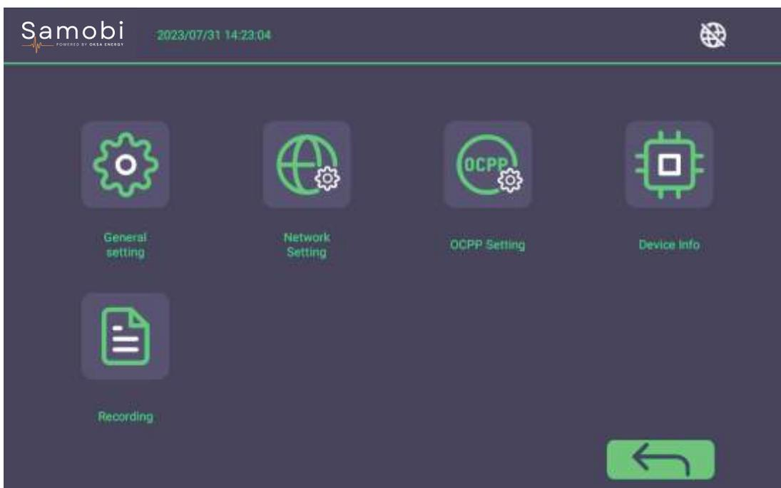
5. General Settings are divided into System Settings, User Preferences, Charging Station Configuration, and Charging connector Configuration.
